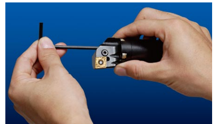
3. 3本のボルトを締めて取付ける Tighten three screws to clamp the boring head.
