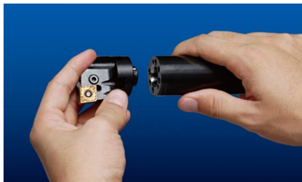
2. 穴位置を合わせる Align the boring head with the installing position.
