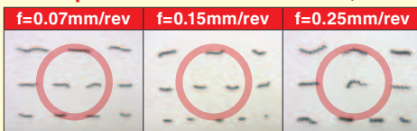
PP Chipbreaker controls chips stability at high feed rate.
