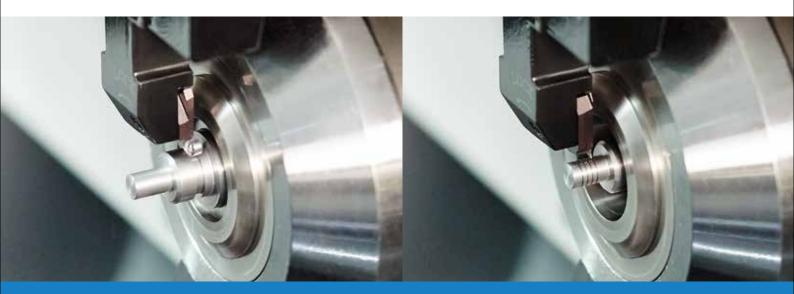
Low Cutting Force with a Large Rake Angle. High Precision Grooving
